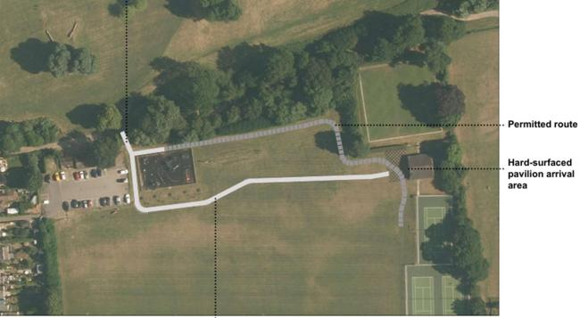
HDA Recommended Route: 1.5m Trailfex path to tie-in with proposed car park upgrade; avoids tree roots, retains existing desire lines, and provides a most direct path across the recreation area.
