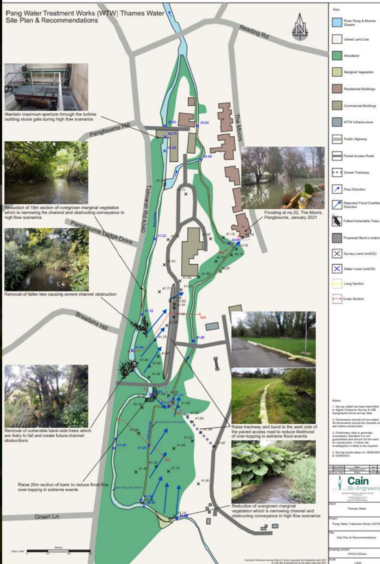
Figure 5. PR14533_103_wsc_Pang WTW - Site Plan & Recommendations V2.
